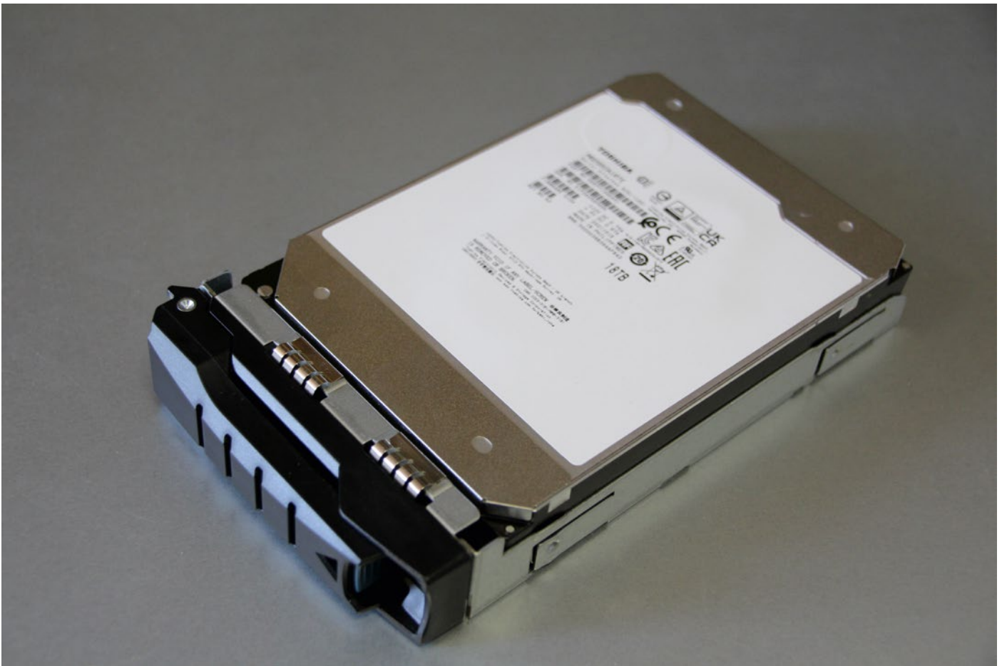
Picture 2: Toshiba HDD MG09SCA18TE in JBOD tray.
