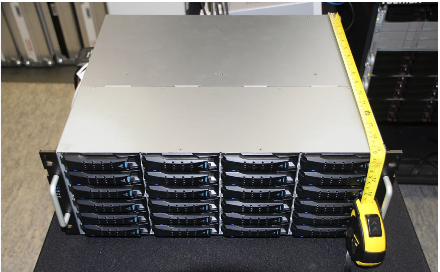
Picture 1: JBOD in the Toshiba lab
