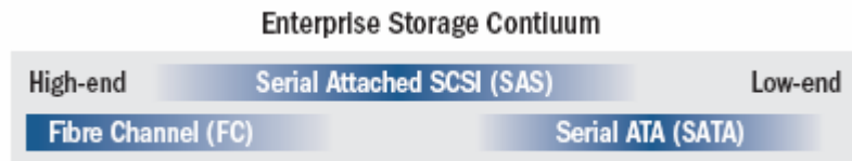
Figure 5: SAS will become the technology of choice for most storage needs, while coexisting with FC and SATA for very high end, or very cost-conscious requirements.
